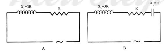
Calculate the ratio of power factor of the circuit B to the power factor of circuit A.
